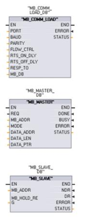
The MB\_COMM\_LOAD instruction configures a port on the CM module for Modbus RTU protocol communications. You can use either the RS232 or the RS485 CM module. Your user program must execute the MB\_COMM\_LOAD to configure a port before either a MB\_SLAVE or a MB\_MASTER instruction can communicate with that port.
