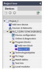
Your program code consists of instructions that the PLC executes in sequence. For this example, you use ladder logic (LAD) to create the program code. The LAD program is a sequence of networks that resemble the rungs of a ladder.
