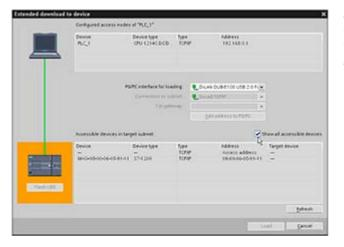
After completing the configuration, download the project to the CPU. The IP address for the CPU and for the router (if applicable) are configured when you download the project.
