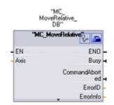
MC\_MoveRelative starts a positioning motion relative to the start position.
