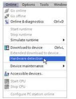
If you are connected to a CPU, you can upload the configuration of that CPU, including any modules, to your project. Simply create a new project and select the "unspecified CPU" instead of selecting a specific CPU. (You can also skip the device configuration entirely by selecting the "Create a PLC program" from the "First steps". STEP 7 Basic then automatically creates an unspecified CPU.)
