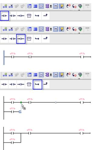
Use the buttons on the "Favorites" to insert contacts and coils onto the network:
