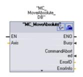
MC\_MoveAbsolute starts motion to an absolute position. The job ends when the target position is reached.
