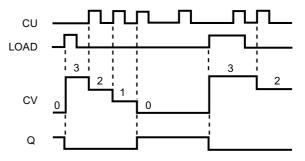
The CTUD counts up or down by 1 on the 0 to 1 transition of the Count up (CU) or Count down (CD) inputs. The figure shows a CTUD timing diagram with an unsigned integer count value (where PV = 4).
