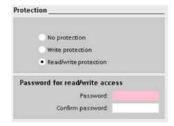
The CPU provides 3 levels of security for restricting access to specific functions. When you configure the security level and password for a CPU, you limit the functions and memory areas that can be accessed without entering a password.
