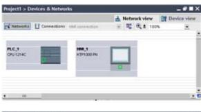
Select "Network view" to display the devices to be connected.
