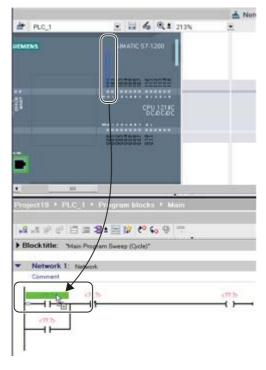
To help you perform tasks quickly and easily, STEP 7 Basic allows you to drag and drop elements from one editor to another. For example, you can drag an input from the CPU to the address of an instruction in your user program. (You must zoom in at least 200% to select the I/O of the CPU.)
