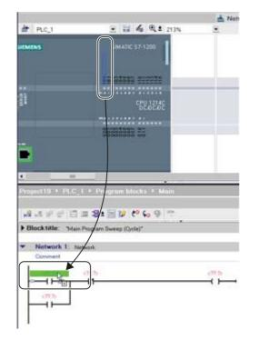
You can also drag the I/O addresses directly from the CPU. Simply split the work area of the Project view (Page 17).
