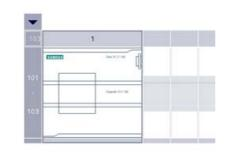
From the device configuration editor, you select the option for detecting the configuration of the connected device.
